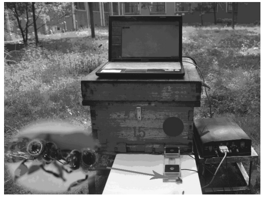
图1 蜜蜂 RFID 记录系统包括电子标签、天线和阅读器 Fig. 1 Radio frequency identification (RFID) system including electronic chips, antennae and reader.
